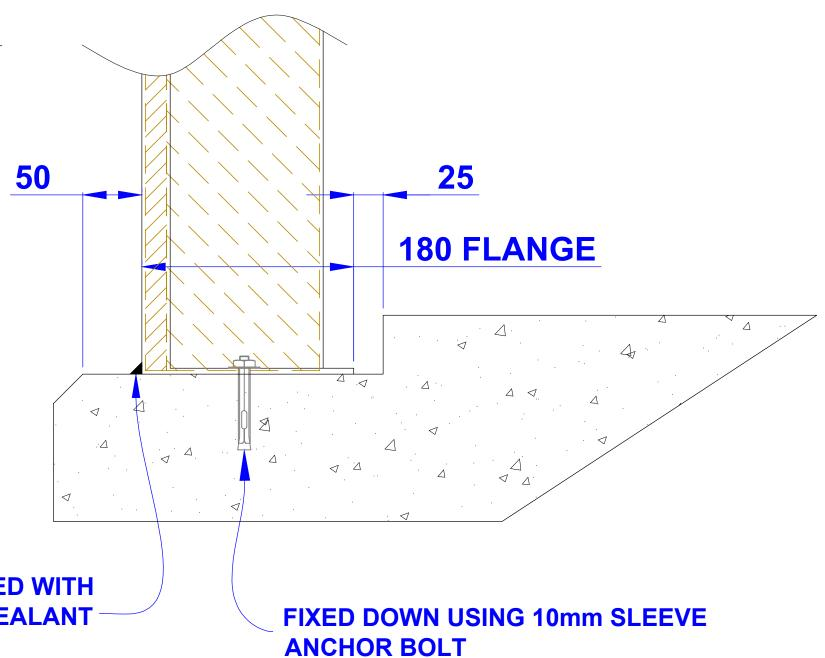
**PERIMETER SEALED WITH SILICONE SEALANT**
