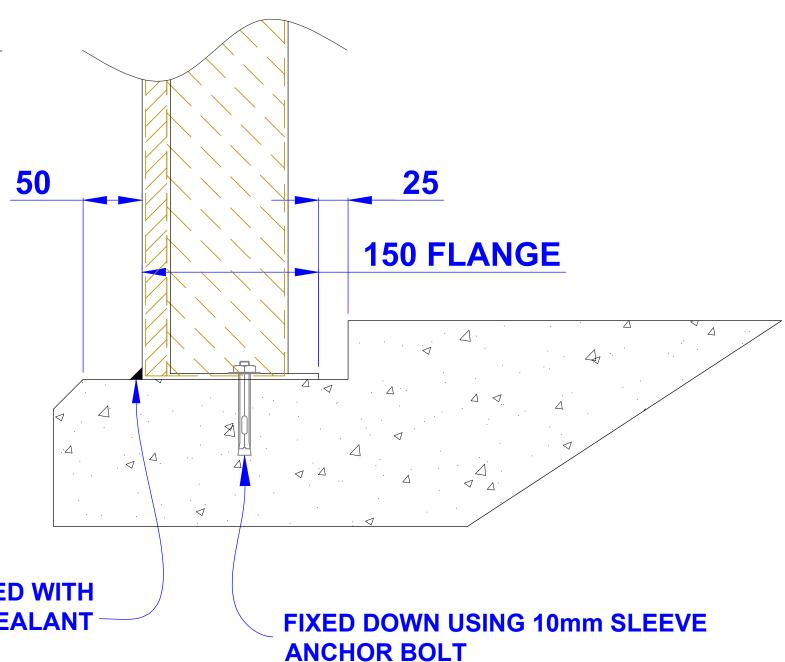
**PERIMETER SEALED WITH SILICONE SEALANT**
