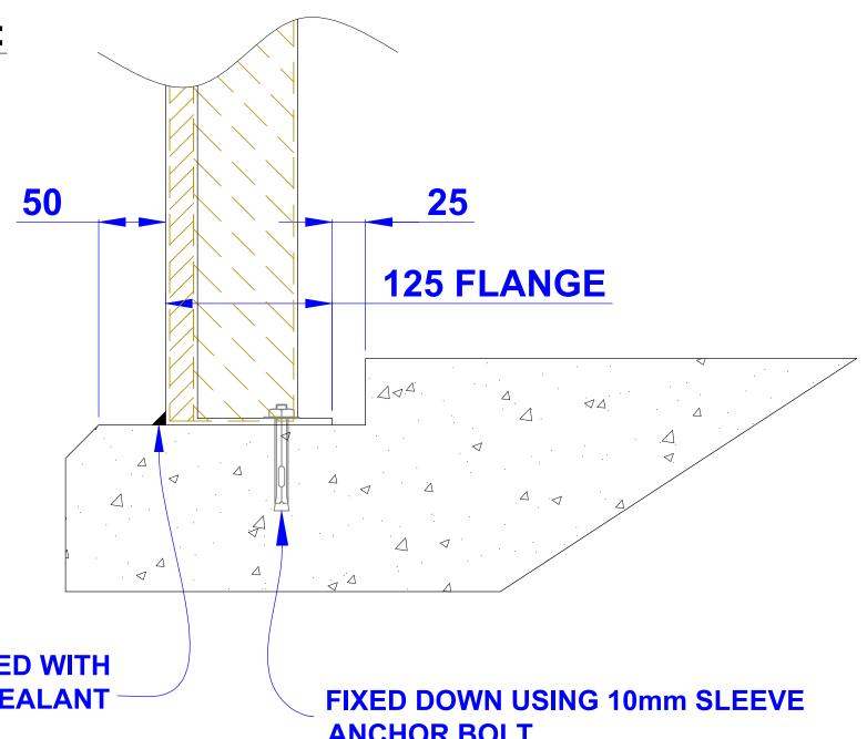
PERIMETER SEALED WITH **SILICONE SEALANT**
